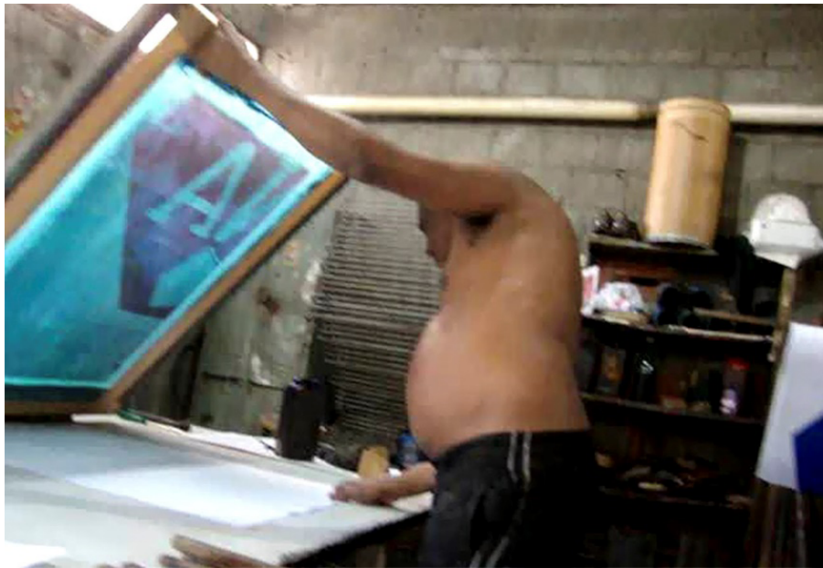
Figure 3. Screen printing process in Baranda's workshop.
