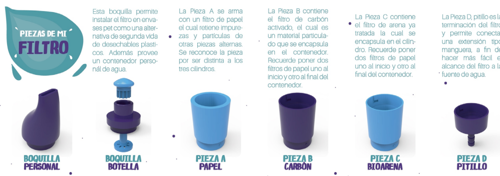
Source: FabLab Nariño (2019). Figure 9. Parts of the AcuaLab Filter.
