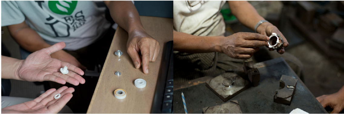
Figure 22. 3D-printed spacer rings for Proximity Designs.
